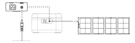
A Solar panel can be used to charge the power station as shown in the above diagram
