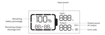
Battery capacity: When the power station is being charged, the SOC icon will flicker.
