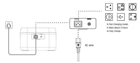
Please use the standard AC charging Cable for fast charging. AC Charging Cable should directly plug into 10A (or above) wall-mounted socket. We take no responsibilities for any damage caused by using unofficial AC charging cable, and other failures to follow instructions.
